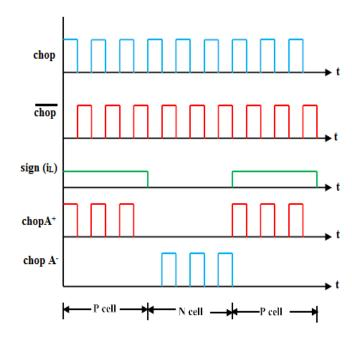
Fig. 5. Signals for PWM generator.
