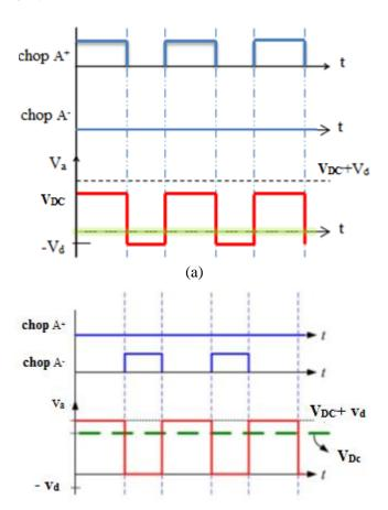
Fig. 8. Terminal voltage and PWM control signals without dead time. (a) iL > 0. (b) iL < 0.
