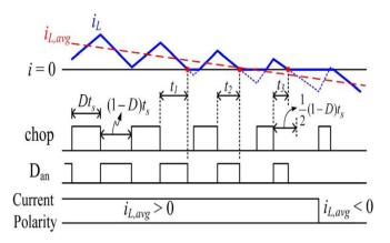
Fig. 9. Load current with several crossing points around zero-current area.
