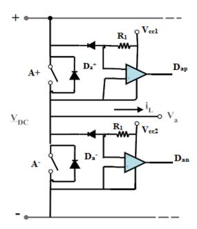
Fig. 6. Previous detection circuit [3]
