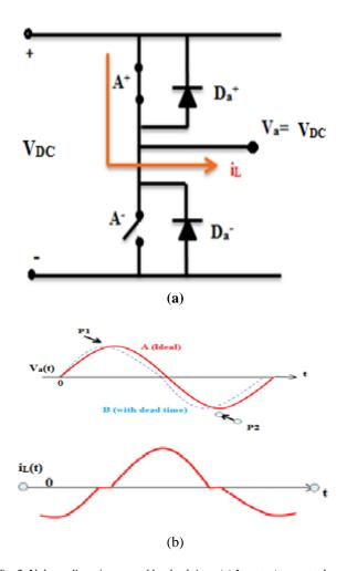
Fig. 2. Voltage distortion caused by dead time. (a) Inverter/converter leg. (b) Voltage distortion caused by dead time.
