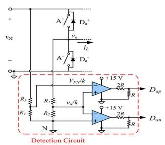
Fig. 7. Proposed detection circuit.
