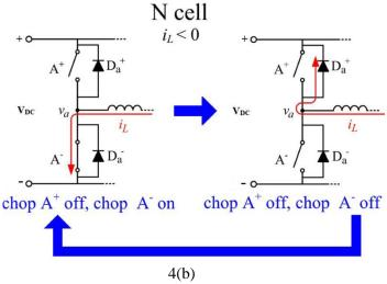
Fig. 4. PWM control based upon P cell and N cell. (a) P-cell control, iL > 0. (b) N-cell control, iL < 0.
