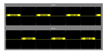
Fig. 11. Gate pulses without dead-time
